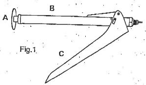
(B) until resistance is felt. The handle will not touch the barrel. DO NOT apply excessive force or the threads will be stripped. Release handle (C) and pull knob (A) completely out, this will release pull-up stud from the insert.
