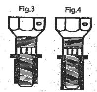
CLOSED END INSERT: (Fig.4) Insert should be threaded onto the pull-up stud until end of stud is even with insert, then insert needs to be turned back one complete turn so insert extends beyond pull-up stud.
